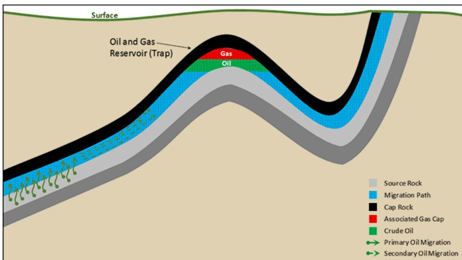
[Cross section of rock layers in a typical oil and gas reservoir](#)<sup>19</sup>
