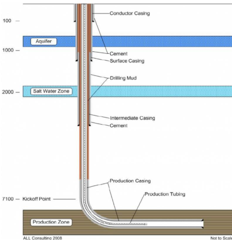
[Cross section of oil well casing](#)<sup>27</sup>
